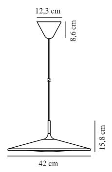
Voltage (V): 230 Volt IP degree: IP20 Class (Class 1, Class 2, Class 3): Class 2 (Double isolated) Socket type: LED Module Dimmerable: True
