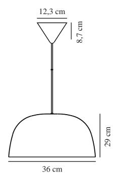
Voltage (V): 230 Volt IP degree: IP20 Maximum bulb wattage (W): 60 Class (Class 1, Class 2, Class 3): Class 2 (Double isolated) Socket type: E27
