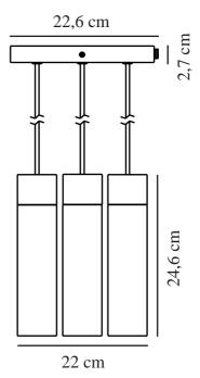
Voltage (V): 230 Volt IP degree: IP20 Maximum bulb wattage (W): 15 Class (Class 1, Class 2, Class 3): Class 2 (Double isolated) Socket type: GU10
