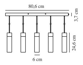
Voltage (V): 230 Volt IP degree: IP20 Maximum bulb wattage (W): 15 Class (Class 1, Class 2, Class 3): Class 2 (Double isolated) Socket type: GU10
