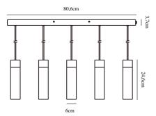
Voltage (V): 230 Volt IP degree if the fixture includes two types of IP degree: IP20 Class (Class I, Class II, Class III): Class 2 (Double isolated) Lampholder type (eg, E27/E14, etc): GU10
