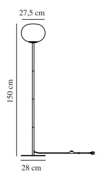
IP degree: IP20 Maximum bulb wattage (W): 25 Class (Class 1, Class 2, Class 3): Class 2 (Double isolated) Socket type: E27
