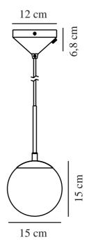
Voltage (V): 220-240 Volt IP degree: IP20 Maximum bulb wattage (W): 10 Class (Class 1, Class 2, Class 3):
