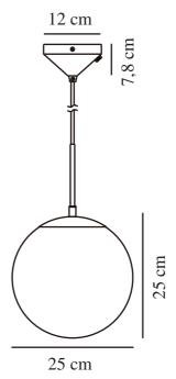
Voltage (V): 220-240 Volt IP degree: IP20 Maximum bulb wattage (W): 15 Class (Class 1, Class 2, Class 3): Class 2 (Double isolated)
