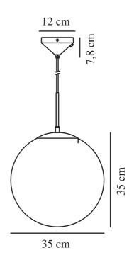
Voltage (V): 220-240 Volt IP degree: IP20 Maximum bulb wattage (W): 15 Class (Class 1, Class 2, Class 3): Class 2 (Double isolated) Socket type: E27 Parallel connection: False
