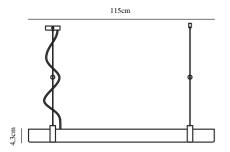
Voltage (V): 230 Volt IP degree if the fixture includes two types of IP degree: IP20 Class (Class I, Class II, Class III): Class 2 (Double isolated) Lampholder type (eg, E27/E14, etc): LED Module Dimmerable: True
