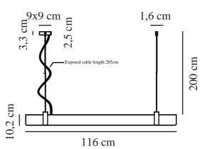
Voltage (V): 220-240 Volt IP degree: IP20 Maximum bulb wattage (W): 28W Class (Class 1, Class 2, Class 3): Class 2 (Double isolated) Socket type: LED - Nonreplaceable light source Dimmerable: True Parallel connection: False
