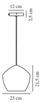
Voltage (V): 230 Volt IP degree: IP20 Maximum bulb wattage (W): 40 Class (Class 1, Class 2, Class 3): Class 2 (Double isolated) Socket type: E27
