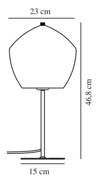
Voltage (V): 230 Volt IP degree: IP20 Maximum bulb wattage (W): 40 Class (Class 1, Class 2, Class 3): Class 2 (Double isolated) Socket type: E27 Switch placement: On the cable
