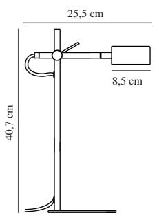
Voltage (V): 220-240 Volt IP degree: IP20 Class (Class 1, Class 2, Class 3): Class 2 (Double isolated) Socket type: LED – Nonreplaceable light source Switch placement: On the cable
