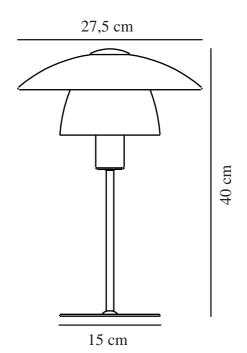
Voltage (V): 230 Volt IP degree: IP20 Maximum bulb wattage (W): 15 Class (Class 1, Class 2, Class 3): Class 2 (Double isolated) Socket type: E27 Switch placement: On the fixture
