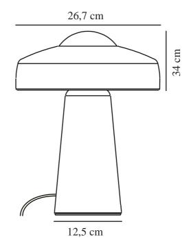
Voltage (V): 230 Volt IP degree: IP20 Maximum bulb wattage (W): 40W Class (Class 1, Class 2, Class 3): Class 2 (Double isolated) Socket type: E27 Switch placement: On the fixture
