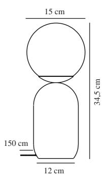
Voltage (V): 220-240 Volt IP degree: IP20 Maximum bulb wattage (W): 25 Class (Class 1, Class 2, Class 3): Class 2 (Double isolated) Socket type: E14 Switch placement: On the cable Parallel connection: False
