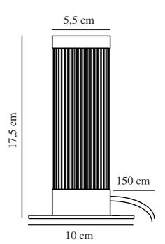
Voltage (V): 230 Volt IP degree: IP20 Maximum bulb wattage (W): 40W Class (Class 1, Class 2, Class 3): Class 2 (Double isolated) Socket type: E27 Switch placement: On the cable
