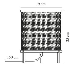
Voltage (V): 230 Volt IP degree: IP20 Maximum bulb wattage (W): 15W Class (Class 1, Class 2, Class 3):
