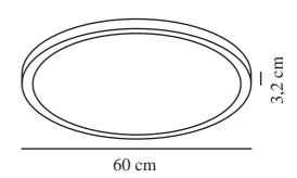
Voltage (V): 220-240 Volt IP degree: IP20 Class (Class 1, Class 2, Class 3): Class 1 (Earth contact) Socket type: LED – Nonreplaceable light source Parallel connection: False
