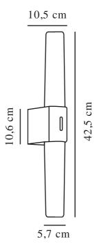
Voltage (V): 230 Volt IP degree: IP44 Class (Class 1, Class 2, Class 3): Class 2 (Double isolated) Socket type: LED – Nonreplaceable light source
