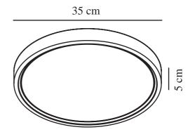
Voltage (V): 230 Volt IP degree: IP44 Class (Class 1, Class 2, Class 3): Class 2 (Double isolated) Socket type: LED - Nonreplaceable light source
