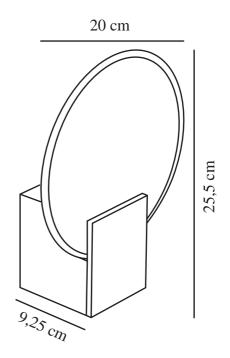
Voltage (V): 230 Volt IP degree: IP44 Class (Class 1, Class 2, Class 3): Class 2 (Double isolated) Socket type: LED – Nonreplaceable light source
