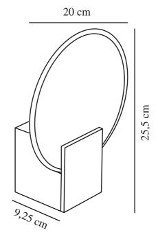
Voltage (V): 230 Volt IP degree: IP44 Class (Class 1, Class 2, Class 3): Class 2 (Double isolated) Socket type: LED – Nonreplaceable light source
