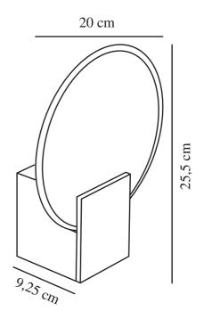
Voltage (V): 230 Volt IP degree: IP44 Class (Class 1, Class 2, Class 3): Class 2 (Double isolated) Socket type: LED Module
