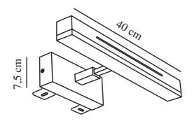
Voltage (V): 230 Volt IP degree: IP44 Class (Class 1, Class 2, Class 3): Class 2 (Double isolated) Socket type: LED Module
