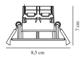
Voltage (V): 220-240 Volt IP degree: IP65 Class (Class 1, Class 2, Class 3): Class 2 (Double isolated) Socket type: LED – Nonreplaceable light source Parallel connection: True
