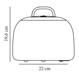
Voltage (V): 5 Volt IP degree: IP65 Class (Class 1, Class 2, Class 3): Class 3 (12V) Socket type: LED – Nonreplaceable light source Dimmerable: True
