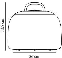
Voltage (V): 3,7 Volt IP degree: IP65 Class (Class 1, Class 2, Class 3): Class 3 (12V) Socket type: LED – Nonreplaceable light source Switch placement: On the fixture Parallel connection: False
