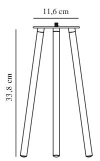
Primary material: Metal Suitable for Seaside: False Colour: Black Height (cm): 33.8 Width (cm): 17.9 Tube Diameter (cm): 1.6 Lenght (cm): 15.7
