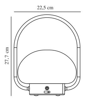
Voltage (V): 5 Volt IP degree: IP65 Class (Class 1, Class 2, Class 3): Class 3 (12V) Socket type: LED – Nonreplaceable light source Dimmerable: True
