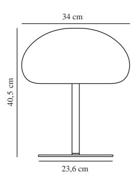
Voltage (V): 5 Volt IP degree: IP65 Class (Class 1, Class 2, Class 3): Class 3 (12V) Socket type: LED – Nonreplaceable light source Dimmerable: True
