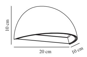
Voltage (V): 220-240 Volt IP degree: IP54 Class (Class 1, Class 2, Class 3): Class 1 (Earth contact) Socket type: LED – Nonreplaceable light source
