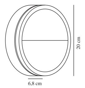
Voltage (V): 220-240 Volt IP degree: IP54 Class (Class 1, Class 2, Class 3): Class 1 (Earth contact) Socket type: LED – Non-
