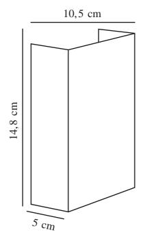
Voltage (V): 220-240 Volt IP degree: IP54 Class (Class 1, Class 2, Class 3): Class 1 (Earth contact) Socket type: LED Module
