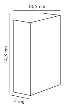
Voltage (V): 230 Volt IP degree: IP54 Class (Class 1, Class 2, Class 3): Class 1 (Earth contact) Socket type: LED – Nonreplaceable light source Parallel connection: True
