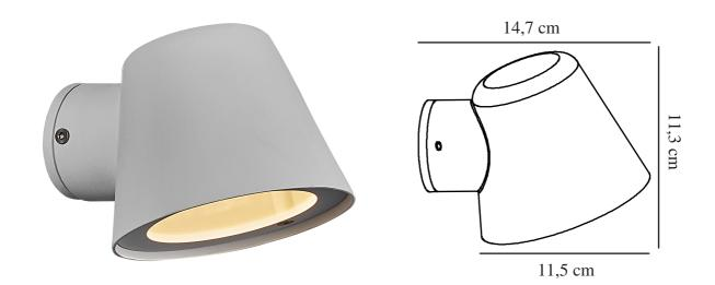
Voltage (V): 230 Volt IP degree: IP44 Maximum bulb wattage (W): 35W Class (Class 1, Class 2, Class 3): Class 1 (Earth contact) Socket type: GU10 Parallel connection: False
