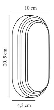
Voltage (V): 230 Volt IP degree: IP54 Class (Class 1, Class 2, Class 3): Class 2 (Double isolated) Socket type: LED - Nonreplaceable light source
