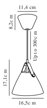
Voltage (V): 230 Volt IP degree: IP20
