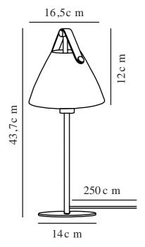
Voltage (V): 230 Volt IP degree: IP20 Maximum bulb wattage (W): 25W Class (Class 1, Class 2, Class 3): Class 2 (Double isolated) Socket type: G9 Switch placement: On the cable
