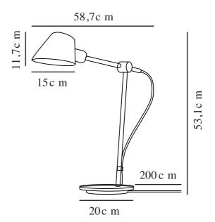
IP degree: IP20 Maximum bulb wattage (W): 60W Class (Class 1, Class 2, Class 3): Class 2 (Double isolated) Socket type: E27
