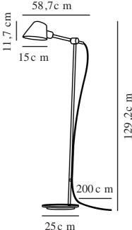
Voltage (V): 230 Volt IP degree: IP20 Maximum bulb wattage (W): 60 Class (Class 1, Class 2, Class 3): Class 2 (Double isolated) Socket type: E27 Switch placement: On the fixture
