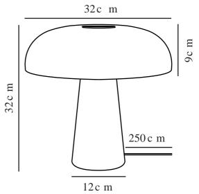
Voltage (V): 220-240 Volt IP degree: IP20
