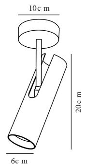
Voltage (V): 220-240 Volt IP degree: IP20 Maximum bulb wattage (W): 8 Class (Class 1, Class 2, Class 3): Class 2 (Double isolated) Socket type: GU10 Parallel connection: False
