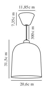
Voltage (V): 220-240 Volt IP degree: IP20 Maximum bulb wattage (W): 25 Class (Class 1, Class 2, Class 3): Class 2 (Double isolated) Socket type: E27 Dimmerable: Yes with compatible bulb Parallel connection: False
