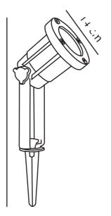
Voltage (V): 230 Volt IP degree: IP54 Maximum bulb wattage (W): 35 Class (Class 1, Class 2, Class 3): Class 1 (Earth contact) Socket type: GU10 Parallel connection: False
