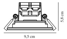
Voltage (V): 230 Volt IP degree: IP44 Class (Class 1, Class 2, Class 3): Class 2 (Double isolated) Socket type: LED - Nonreplaceable light source Parallel connection: True
