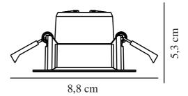
Voltage (V): 230 Volt IP degree: IP20 Class (Class 1, Class 2, Class 3): Class 2 (Double isolated) Socket type: LED – Nonreplaceable light source Parallel connection: True
