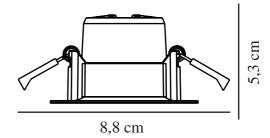
Voltage (V): 230 Volt IP degree: IP20 Class (Class 1, Class 2, Class 3): Class 2 (Double isolated) Socket type: LED Module Parallel connection: True
