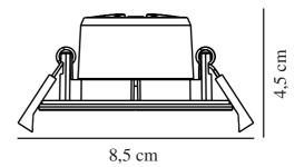
Voltage (V): 230 Volt IP degree: IP65 Class (Class 1, Class 2, Class 3): Class 2 (Double isolated) Socket type: LED - Nonreplaceable light source Parallel connection: True
